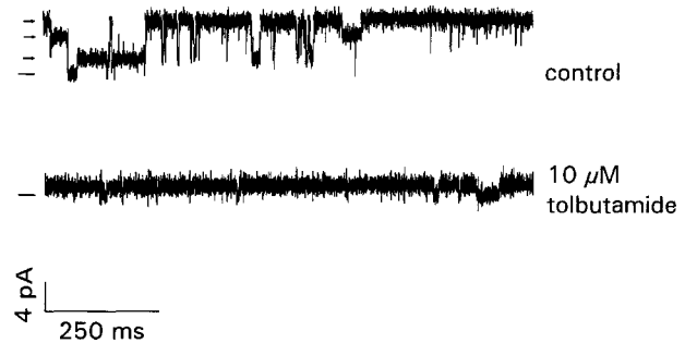
Fig. 8. The effect of tolbutamide on the ATP-inhibited K + channel and on a 30 pS channel. Recordings in the inside-out configuration in symmetrical 120 mM K + solution at a holding potential of -60 mV. The upper recording shows one 30 pS and one ATP-inhibited K + channel in the absence of tolbutamide (control). The bar indicates the closed state, the arrows (beginning at the closed state) the open state of the 30 pS channel, of the ATP-inhibited K + channel and of both channels simultaneously. Tolbutamide (10 μM) irreversibly blocks the ATP-inhibited K + channel 6 min after application, whereas the 30 pS channel remains unaffected (lower recording).
